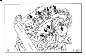
(d) Using SST, loosen the injection pipe unions of common rail side.
