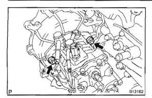
(c) Remove the 2 nuts and supply pump.
