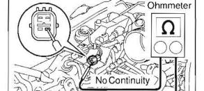
(c) Using an ohmmeter, check that there is no continuity between the injector terminal and ground as shown.
