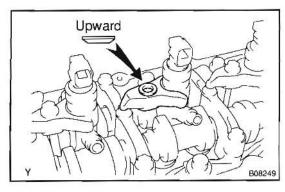
(k) Set the washer on the nozzle holder clamp as shown in the illustration.
