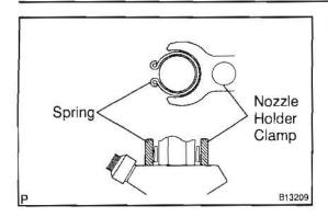
(j) Set the spring to each injector as shown in the illustration.
