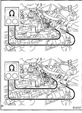
(c) Using an ohmmeter, check that there is no continuity between the terminal and ground as shown.
