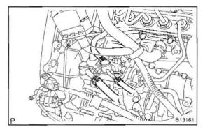
(b) Disconnect the 3 fuel hoses from the supply pump.
