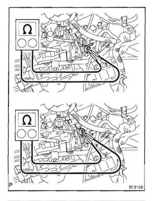
(b) Using an ohmmeter, measure the resistance between terminals as shown.
